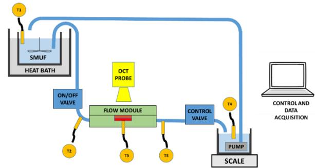
Fig. 1. Schematic drawing of the measurement setup.
