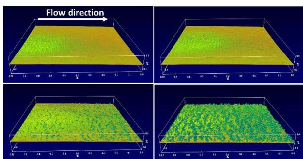
Fig. 9. OCT images from a run at flow rate 300 ml/min. Times of the image are start of SMUF flow, after two hours, after three hours, and after 7.5 hours.
