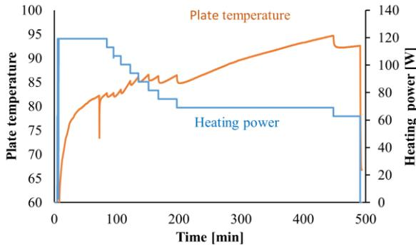
Fig. 5. The heating power and the temperature of the heating element during the experiment that resulted in the deposited layer shown in Fig. 4.
