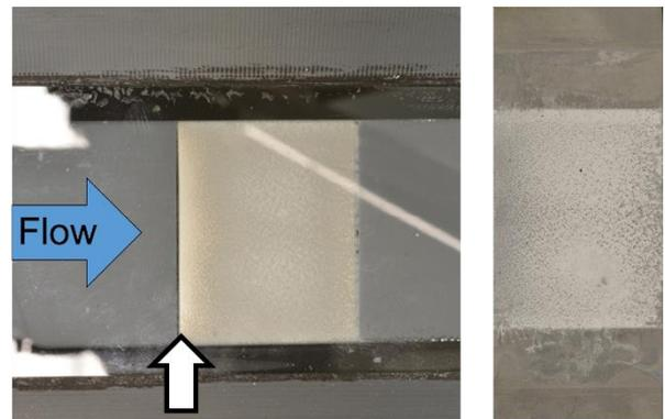
Fig. 4. An example of a deposited layer on the target plate. The left image is taken during the experiment, the right image after the plate was detached from the module. The vertical arrow marks the leading edge of the plate where the fouling layer is thin.
