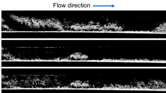
Fig. 6. A set of 2D OCT snapshots (OCT B-scans), from a measurements with dynamic fouling. The width and the height of the images are 8 mm and 1.2 mm, respectively, and the time difference between the images is ten minutes.
