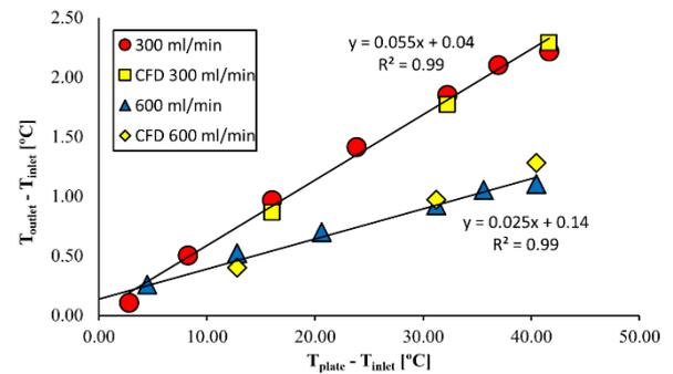
Fig. 3. Heating tests with water and comparison with CFD (Ojaniemi *et. al.* 2019).
