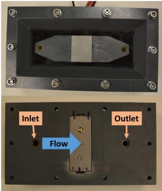
Fig. 2. The flow module assembled (top), and the top half removed (bottom). The dimensions of the flow channel are 140 mm in length, 40 mm in width, and 2 mm in thickness.
