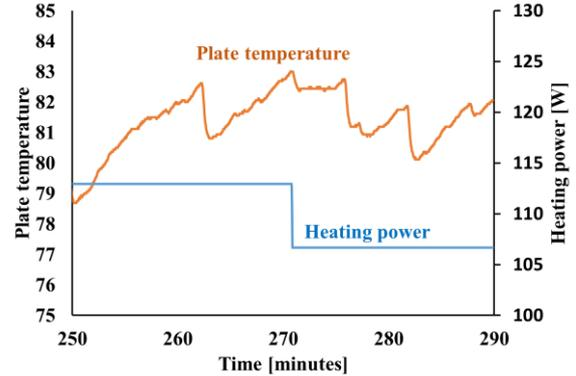
Fig. 7. Dynamic fouling shown in Fig. 6 is visible in the measured temperature data as sharp drops (detachment) and gradual increase to the original value (refouling).
