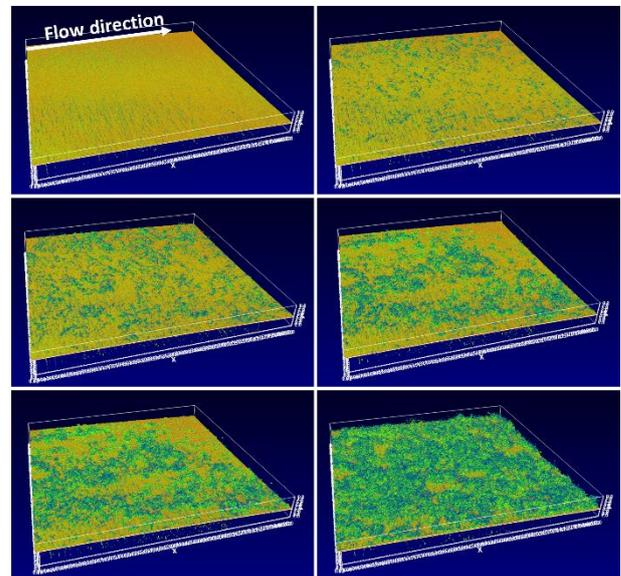
Fig. 8. OCT images of the target plate surface during 5 hours long measurement at flow rate 300 ml/min. The yellow color shows the target plate surface and the green color the deposited layer. The top left image is the starting point of the SMUF flow and the time of the rest of the images are (from left to right and from top to down) 105 minutes, 120 minutes, 150 minutes, 180 minutes, and 300 minutes.
