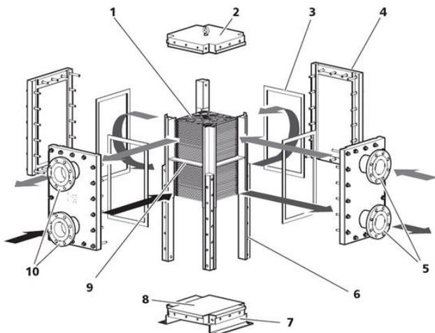
Fig. 2 GEABloc welded plate heat exchanger reboiler. 1 Plate pack, 2 Top head, 3 Panel gasket, 4 Panel, 5 Primary side connection, 6 Column, 7 Support, 8 Bottom head, 9 Baffle/guide plate, 10 Secondary side connection. (GEA Ecoflex GmbH)
