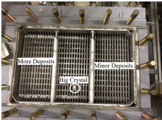
Fig. 3 Deposits formed on the heat exchanger plate pack.
