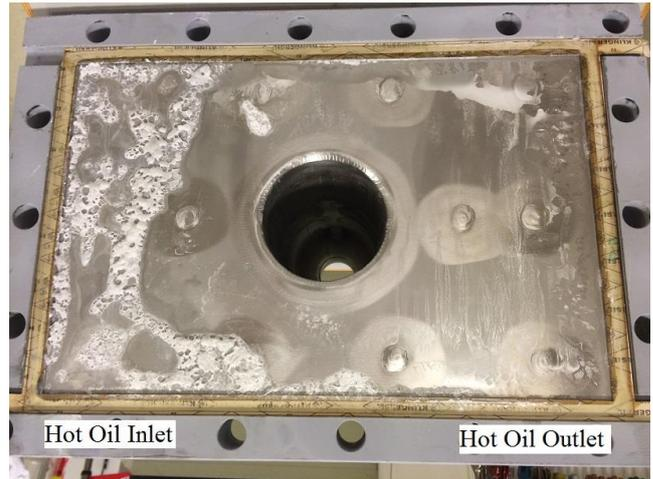
Fig. 4 Deposits formed on the heat exchanger panel.
