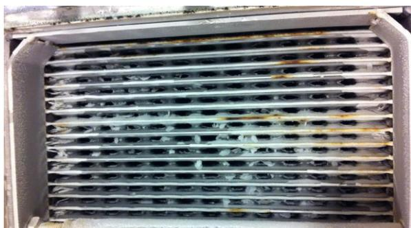
Fig. 6 Deposits formed on the heat exchanger plate pack after MEG solution scaling.
