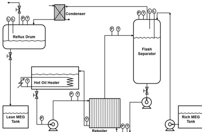
Fig. 1 Process flow diagram for MEG regeneration with PHE reboiler (Fjords Processing AS).
