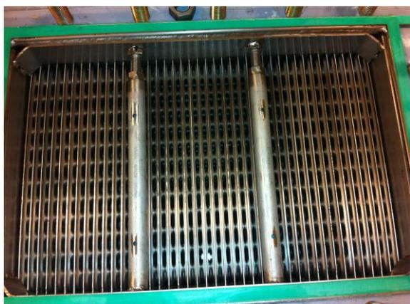
Fig. 7 Heat exchanger plate pack after acid wash.
