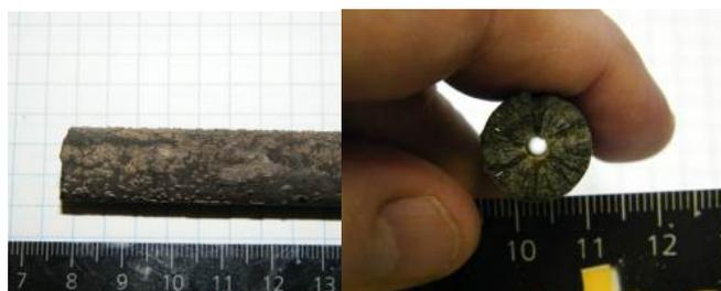
Figure 2. Samples of crystalline deposit (FeCO<sub>3</sub>) removed from a tube side from Lean-Rich amine exchanger.
