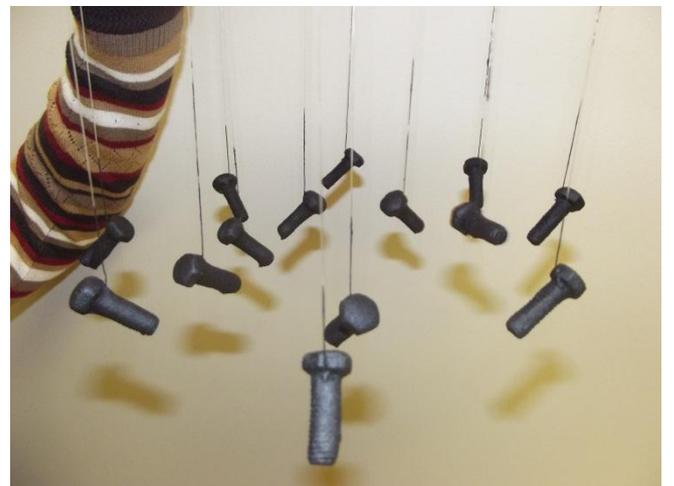
Fig. 7 Test bolts coated in asphalt and suspended by nylon line.
