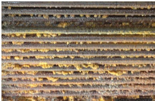
Fig. 2. A fouled straight-tube exchanger with significant fouling between the tubes.
