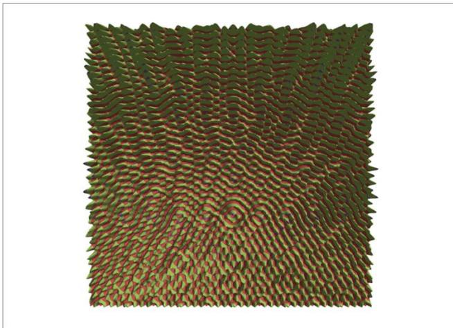
Fig. 6 (b) 11 transducers, spaced at 4 wavelengths, with 180° phase angle, 2D plot
