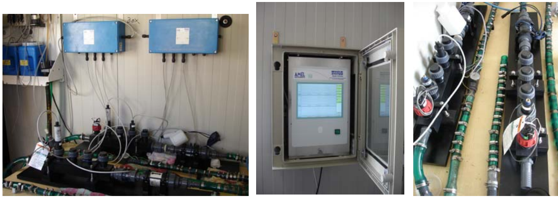
Figure 2: a) View inside of the experimental circuit box (b) the computer display and (c) two hydraulic lines (Control and Treated) with CuNi 70/30 specimens and probes.
