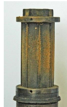
Fig. 13 Photograph of the wired probe after CaSO 4 fouling test; fluid flows clockwise when viewed from the top
