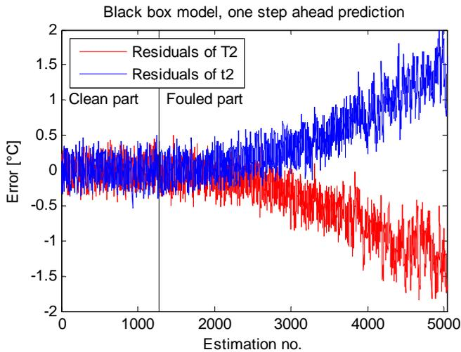
Fig. 8. Plot of the prediction errors for hot and cold output.
