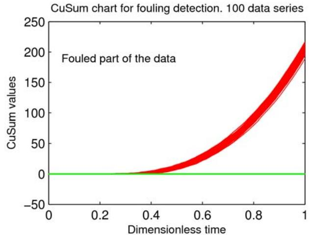
Fig. 7. Drift detection in  $U$  estimated by NTU relations and filtered with empirical relations.
