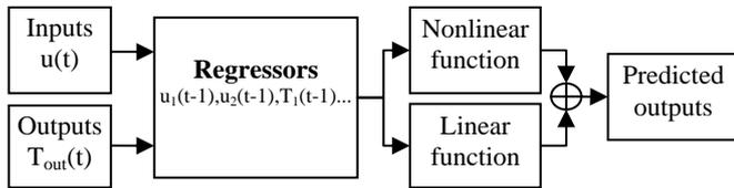
Fig. 2. Block diagram of nonlinear autoregressive model.
