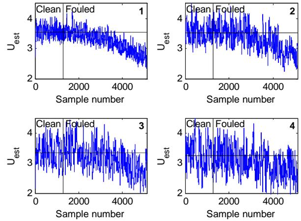
Fig. 1. Estimation of  $U$  from NTU relations on data with different excitement in the inlets.
