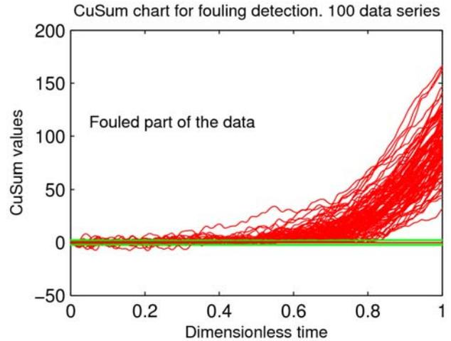
Fig. 6. Drift detection in  $U$  estimated by NTU relations.
