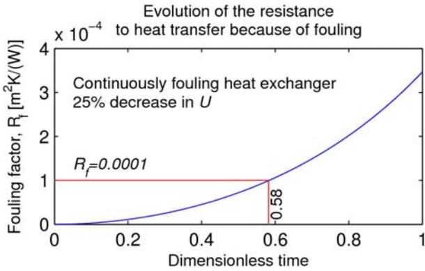
Fig. 4. Evolution of the fouling factor from the time the fouling is initiated.
