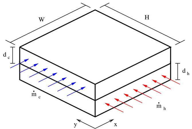
Fig. 3. Graphical layout of the simulated heat exchanger.
