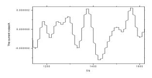
Fig.5 Enlarged picture of the current noise after stainless steel had been immersed in the culture medium which contained SRB for seven days
