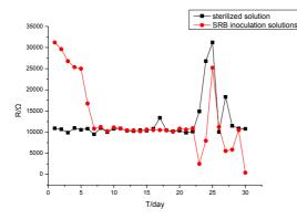
Fig.8 Noise resistance when stainless steel immersed in the culture medium which contained SRB
