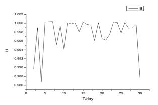
Fig.7 The value of LI when stainless steel immersed in the culture medium which contained SRB
