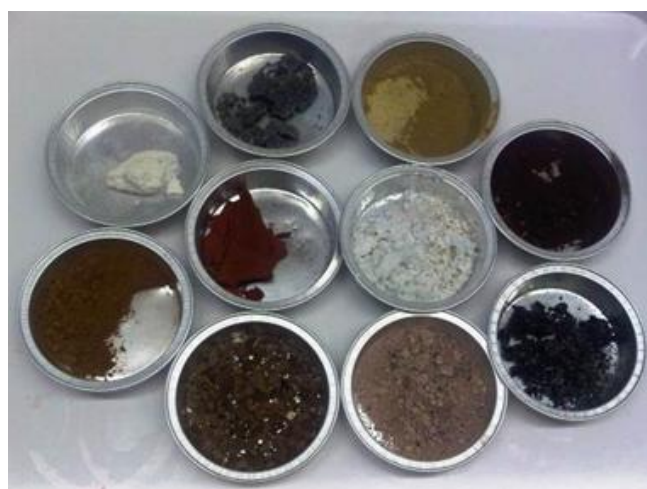
Fig. 4: Deposits found in various systems
