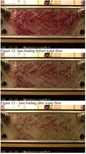
Figure 14 – Jam fouling shortly after ice pig entry
