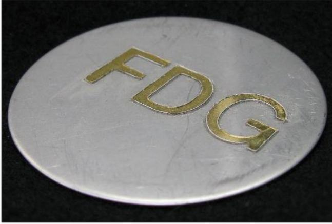
Fig. 7 Patterned 50 mm plate, with ~ 100  $\mu\text{m}$  thick letters.
