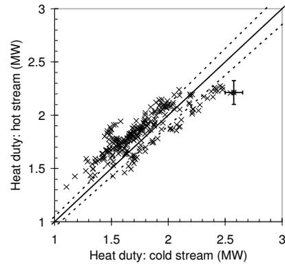
Fig. 4 Calculated duties of hot and cold streams in HEX 9D. Solid line represents of equality and dashed line represents error range generated by Eqs. (12) and (13). Error bar marked on datum indicates uncertainty in data values.
