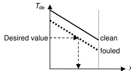
Fig. 2 Schematic of the linearized relationship between desalter inlet temperature and bypass fraction of control HEX.
