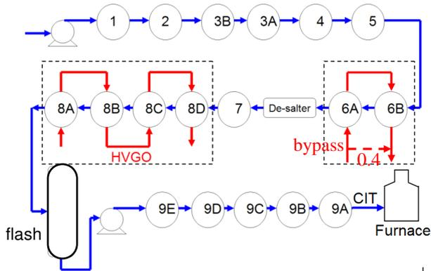
Fig. 3 Case study network consisting of 18 HEXs. CIT is the coil inlet temperature. HEXs 6A, B are used to control the desalter inlet temperature.
