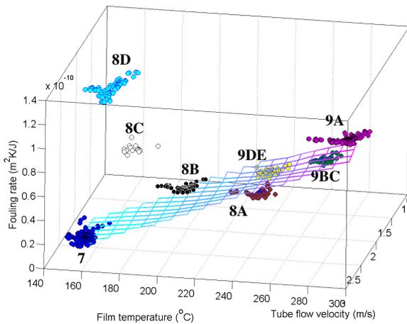
Fig. 5 Comparison of fouling rates in exchangers located downstream of the desalter. The surface indicates the best fit given by the Ebert-Panchal model [Eq. (2)] for the data in HEXs 7, 9A-E. The reported parameters indicate lumped parameter values.
