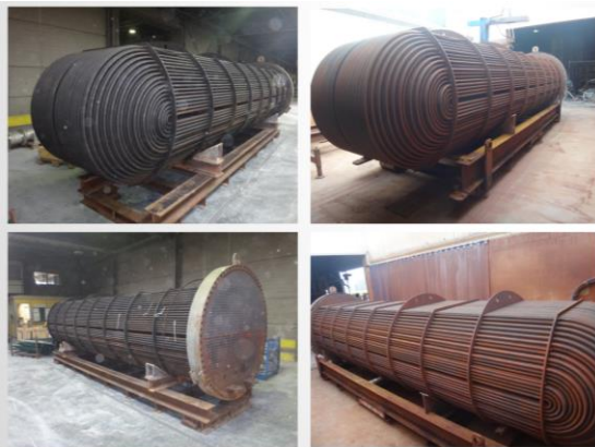
Fig. 15. Thermal cleaning after HP water cleaning.
