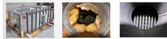
Fig. 9. Cleaning of a compabloc (e.g. polyacryl removal).
