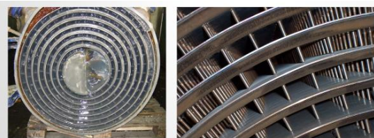
Fig. 8. PE removal from a spiral heat exchanger.
