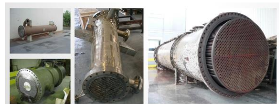
Fig. 6. Different types of bundles with fixed housing.
