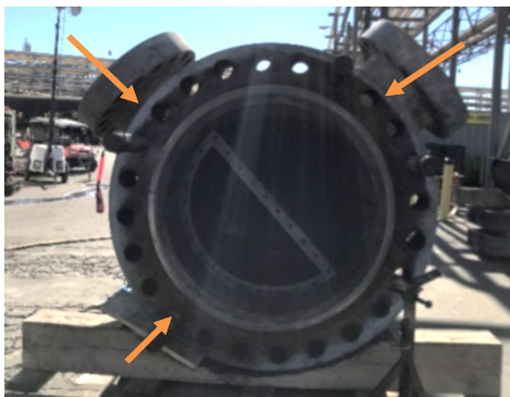
Fig. 8. E-4 Fixed Channel head view showing the layout of the three nozzles on the head at 90°, 180°, and 270°, denoted by the orange arrows.
