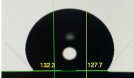
Fig. 6. Sessile contact angle measurement demonstrating hydrophobicity with water on a Minimox coated coupon.
