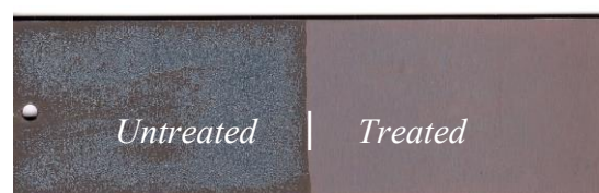
Fig. 1. 410 stainless steel sample, right side treated with Minimox 721 before heat treating. The heat treatment was 1010°C for 30 minutes followed by a 760°C temper, all in air.
