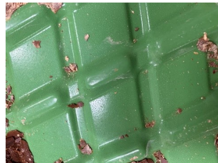
Fig. 8 – Blisters on the 3-layer coating.
