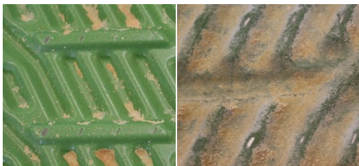
Fig. 16 – Wear at the plate-to-plate contact points on the 3- (left) and 2-layer coating (right).
