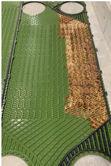
Fig. 7 - Coated plate that was partly cleaned with high water pressure jet. The fouling layer was removed very easily.
