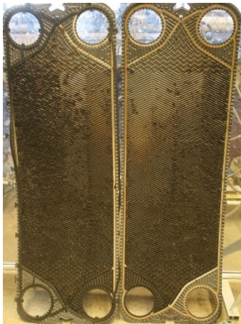
Fig. 21 - Fouling on the plates with coating 2 and the uncoated end plate.
