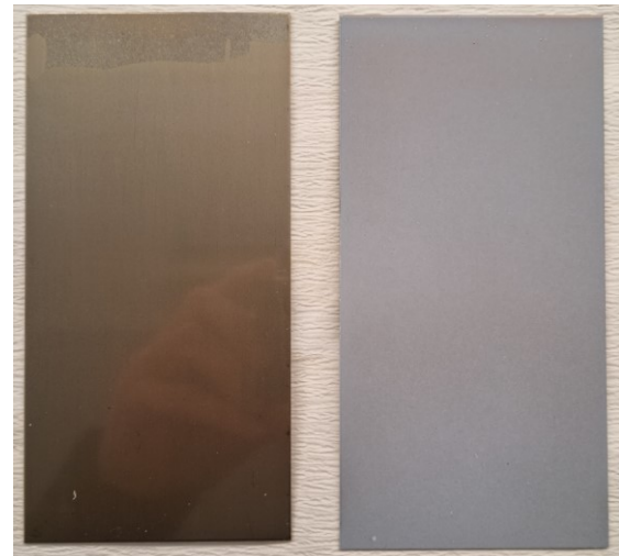
Figure 1: Left coupon: TC200 without added pigments. Right coupon: TC200 with 5% TiO 2
