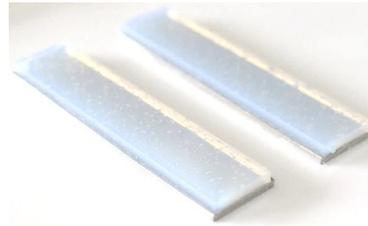
Fig. 1. WPI gel soil attached on a stainless-steel plate as model soil for cleaning investigation.
