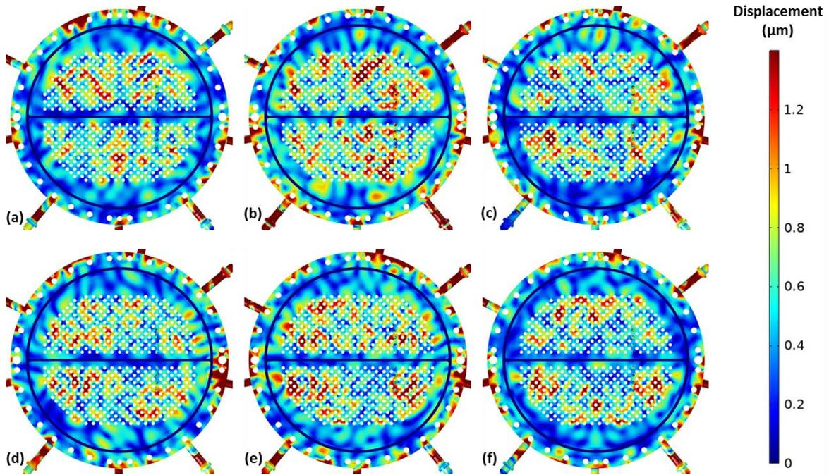
Fig. 6. Ultrasonic displacement field generated in the tubesheet of the large-scale HX
