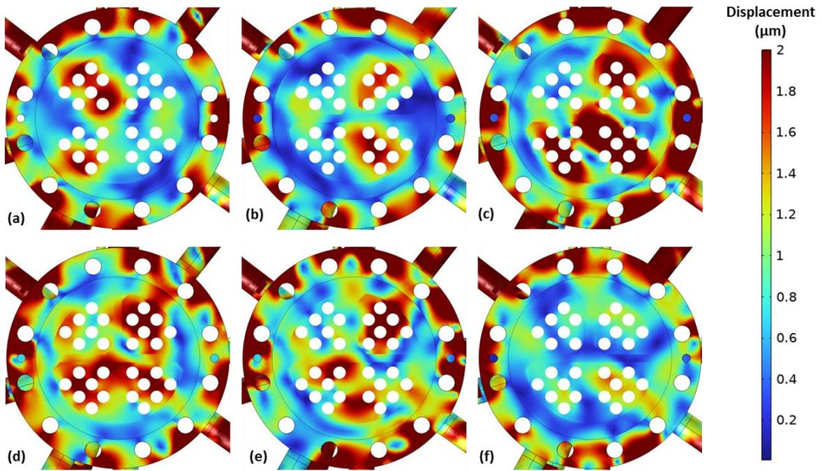
Fig. 4. Ultrasonic displacement field generated in the tubesheet of the small-scale HX
