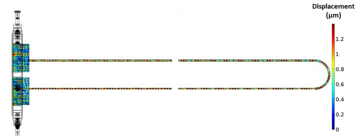
Fig. 7. Ultrasonic displacement field generated in the tubes of the large-scale HX. One of the U tubes is visualized at its entire length, the middle-section of it been excluded to improve the visualization. The field is generated by sonication program setting 1.
