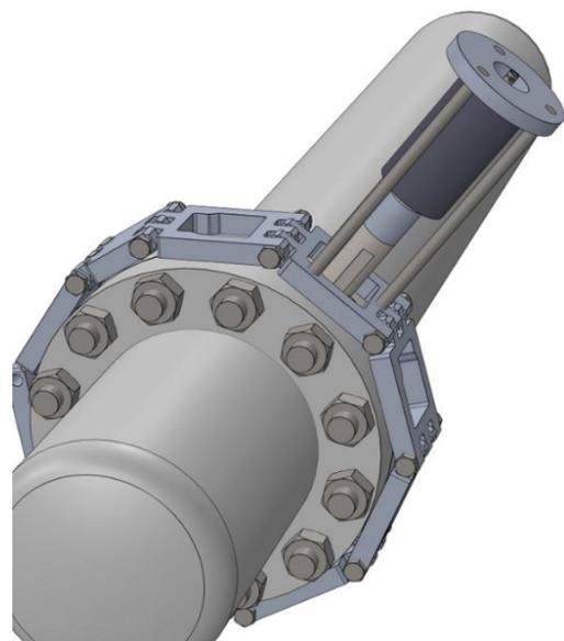
Fig. 2. CAD illustration of the real clamp-on device and the attached ultrasonic transducer with an enclosure.
