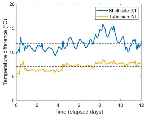
Fig. 8. Temperature differences ( $\Delta T$ ) measured at the shell side (blue) and tube side (yellow) during the fouling prevention run. Both remain nearly constant throughout the trial. Dashed lines represent the related  $\Delta T$  averages.
