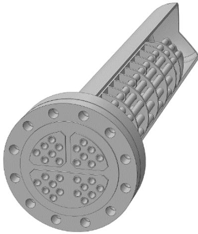
Fig. 3. Internal structure of the small-scale HX model.
