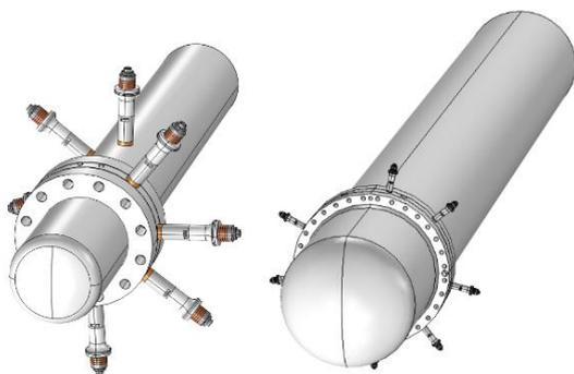
Fig. 1. Simulation geometries: a small-scale U tube HX and a large-scale U tube HX, each sonicated by eight power ultrasound transducers.
