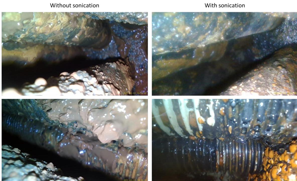
Fig. 9. Borescope images taken after 12 days of HX operation with fouling chemicals. Without sonication (left) and with sonication (right).
