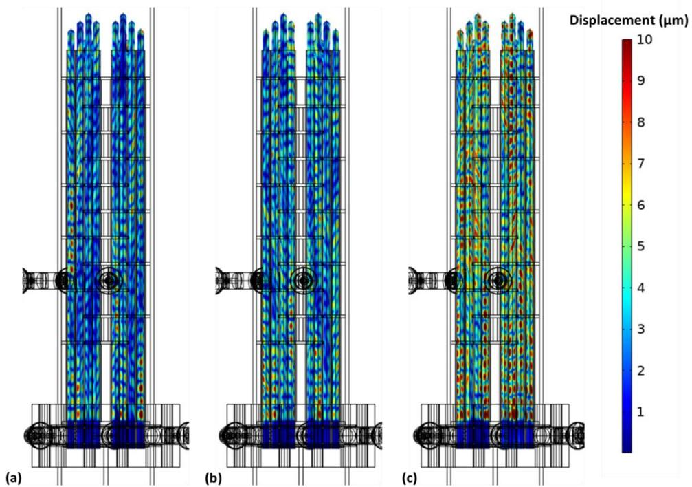
Fig. 5. Ultrasonic displacement field generated in the tubes of the small-scale HX, by sonication program settings (a) 0, (b) 1 and (c) 2.
