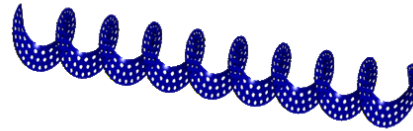
Figure 1 Depiction of a helicoid as used within a continuous helical flow heat exchanger
