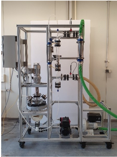
Fig. 3: Photo and flow diagram of the screening apparatus in the configuration of a DN50 column.
