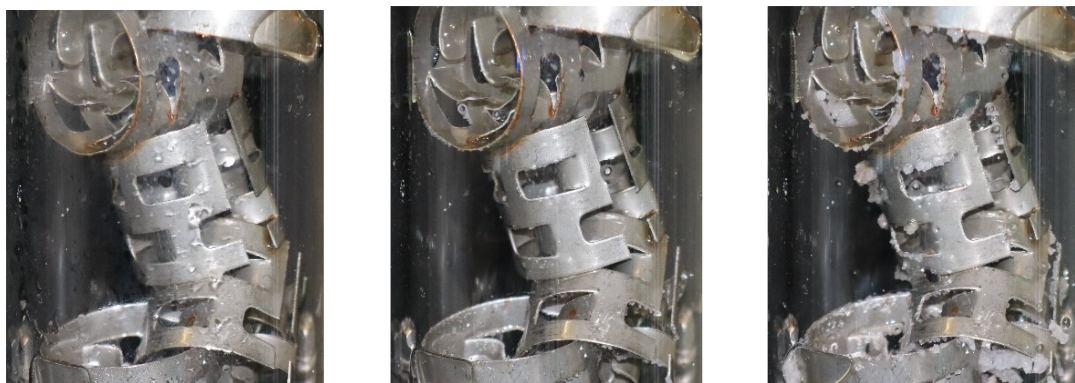
Fig. 4 Fouling on metal Pall-Rings 25 after 0 h, 1 h and 5 h of operation at a liquid load of B = 20 \text{ m}^3/(\text{m}^2 \text{ h}) and gas load of F = 1 \text{ Pa}^{0.5} .
