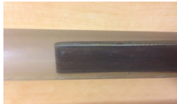
Fig. 4. Pipe with vapor infusion after forty-five days.
