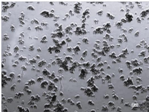
Fig. 4. Asphaltenes in crude, 500X magnification, photo scale L to R is 150 μm
