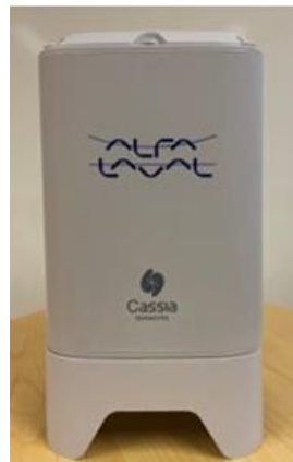
Figure 2: The Alfa Laval gateway for the Smart Heat Exchanger service, provided by Cassia. The limit of the gateway is not in the number of sensor boxes, but the distance to it, recommended up to 50 m.
