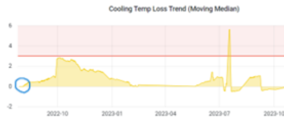
Figure 11: The Temperature Drift output for BatteryX cooling application, showing the cooling temperature loss. The drift is high at 2022.10, when the thermal health trend in figure 9 is at a low, as one would expect.
