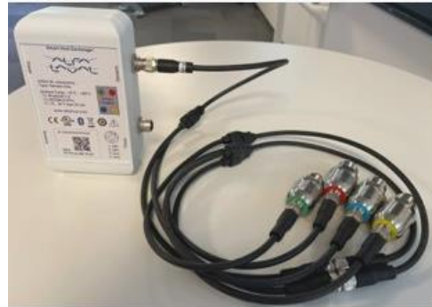
Figure 1: The sensor kit, containing one sensor box and four sensors with cables from WIKA.
