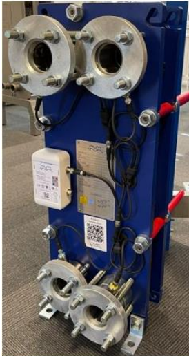
Figure 3: The full installation of the sensor kit on a GPHE in a test-environment.
