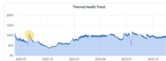
Figure 9: The thermal health trend from 2022.06 – 2024.01. Decline in thermal health indicates deteriorating efficiency of the PHE.
