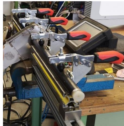
Fig.9. Clamping device for orbital welding
