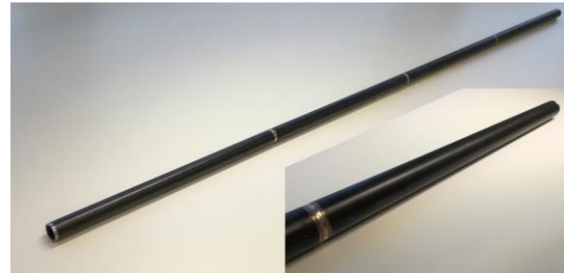
Fig.11. 1.600 mm DLC-coated tube
