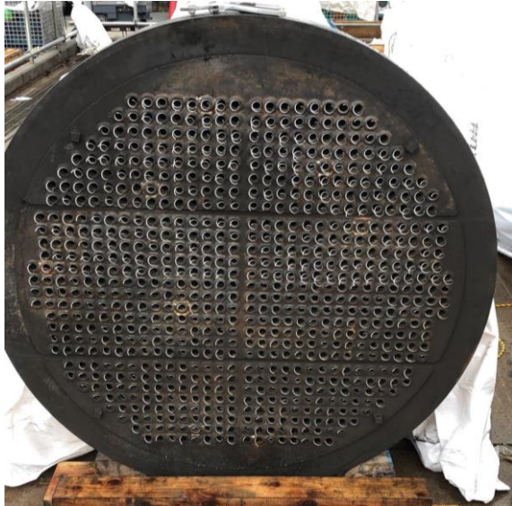
Figure 3 - Photo of the Fixotal devices in the heat exchanger
