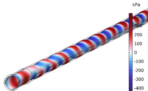
Fig. 4. Temporal snapshot ( t=4 ms) of the simulated acoustic pressure field generated into the water column by a 200W (avg) sonication power.
