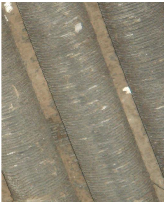
Figure 4: Fouling on open bundle ( T_{2D} = 0.66 )
